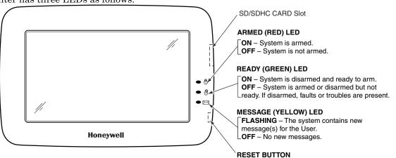
**NOTE:** If the Screen Blackout feature (\*EN50131 Display) is enabled (see below) the keypad returns to the "Home" screen and the "Armed" and "Ready" status LEDs turn OFF after 30 seconds. The keypad will remain in this state until a valid user code is entered.
